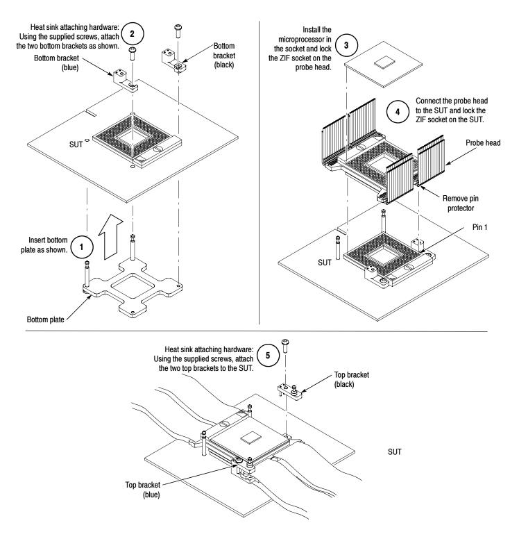
Figure 4: Probe head installation using Chipcool 1 & 2 heat sink hardware
