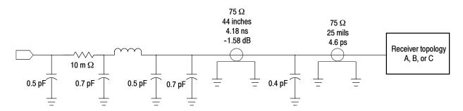
Figure 10: Preprocessor load model for typical signals
