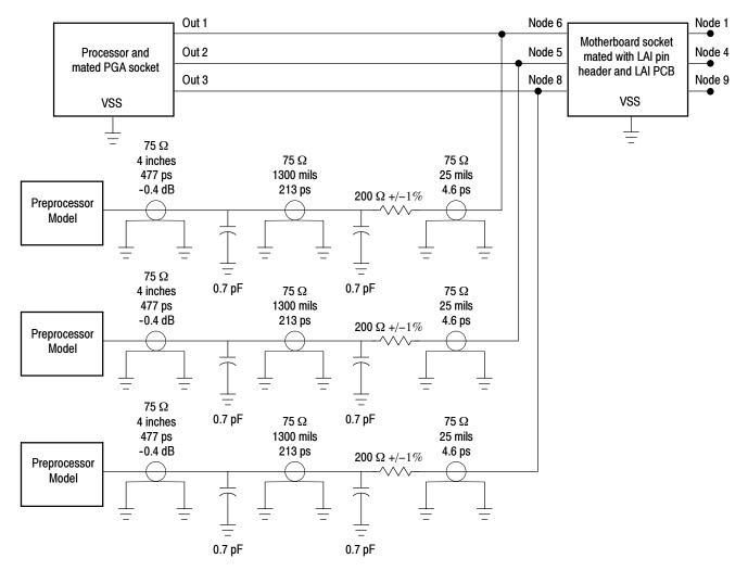
Figure 9: Probe adapter load model for typical signals
