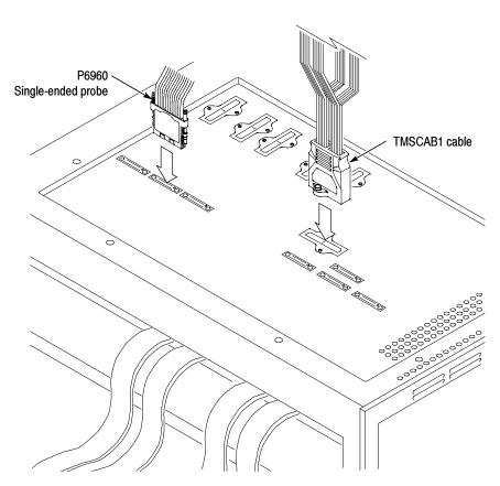
Figure 3: Probe, cable and preprocessor unit
