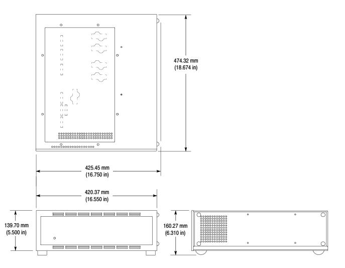
Figure 16: Dimensions of the preprocessor unit
